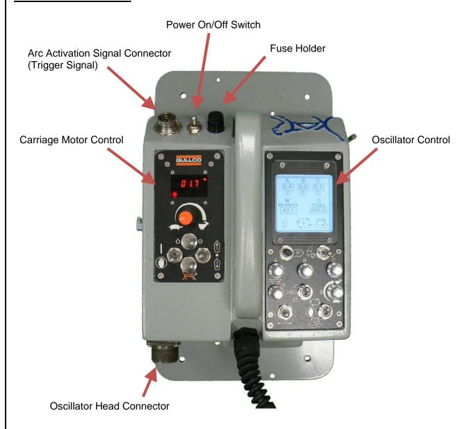
The Power On/Off switch is used to disconnect the power to the rest of the control circuitry.
