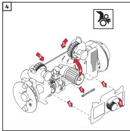
Inserting the wirespool/ basket-type spool
