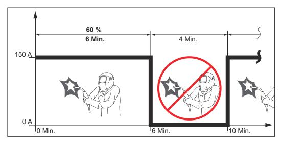
If the device is to be continuously operated without stopping:
