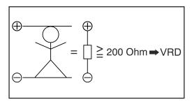
The welding circuit resistance is greater than the minimum human body resistance (greater than or equal to 200 Ohm):
