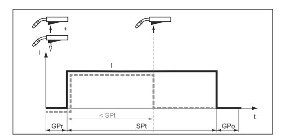
The "Spot welding" mode is suitable for welded joints on overlapped sheets.
