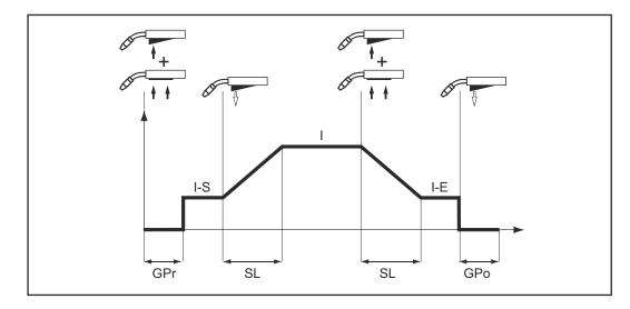
Special 4-step mode allows the starting and final current to be configured in addition to the advantages of 4-step mode.
