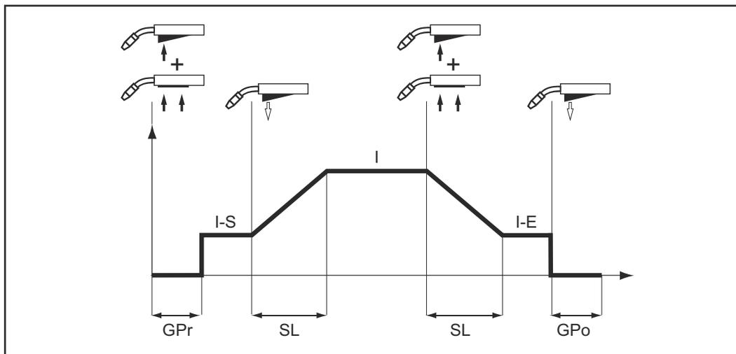
Special 4-step mode allows the starting and final current to be configured in addition to the advantages of 4-step mode.
