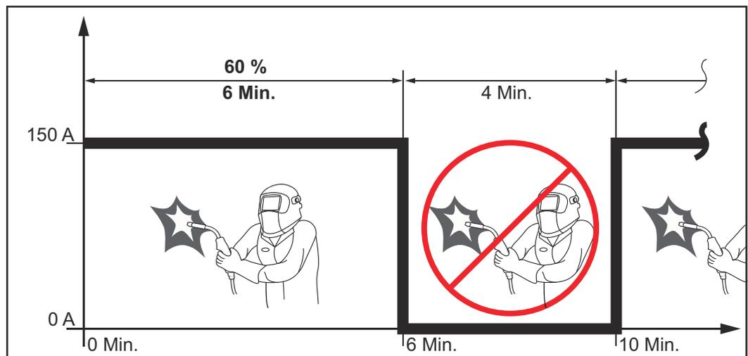
If the device is to be continuously operated without stopping:
