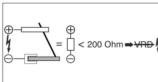
The welding circuit resistance is less than the minimum human body resistance (less than 200 Ohm):
