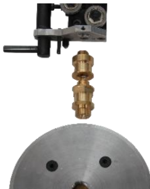
Adapten 9910 0000 54 and 9910 0000 53 for old straighteners with 1/4" thread.
