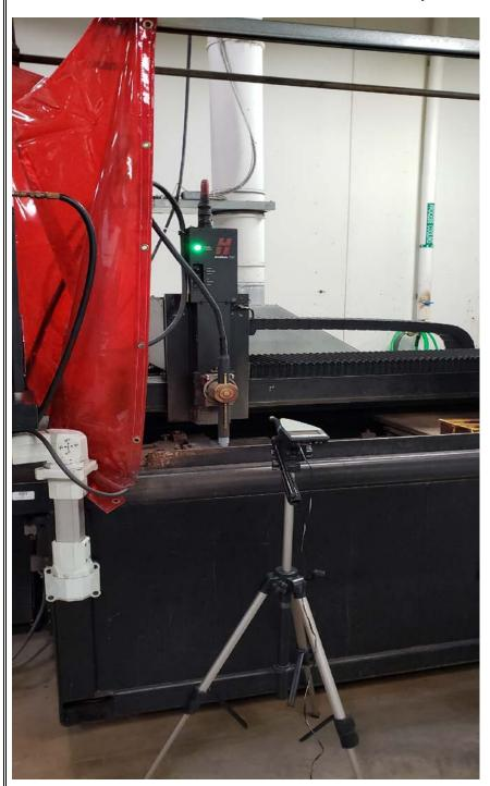
Product Model: Acoustic Measurements for Powermax SYNC Cartridges
