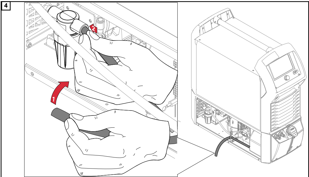
4 Insert the coolant hose into the coolant pre-filter
