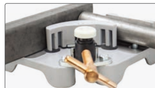
Level parts with screw
