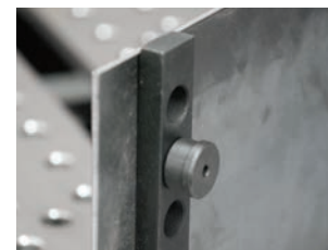
Magnet keeps sheet metal in vertical position
