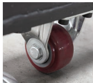
Two casters for quick repositioning of manipulator.
