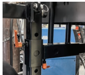
Height adjustment: 50.8 mm Extends: 76.2 mm
